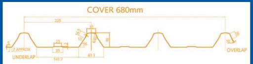
APMAX SPECIFICATIONS Material - High tensile steel, G550 Base metal thickness (B.M.T.) - 0.42/0.48mm
