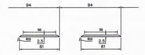
Number of slots per lineal meter of gutter = 10.64 Slot area = 142.5mm²per slot Total front slot opening area = 1567.7mm² per lineal meter of gutter Front slot overflow capacity = 0.63L/s/m
