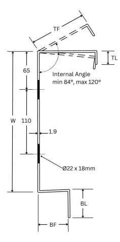
Apex Fascia Purlins are roll-formed from Hi-Tensile Galvanised steel with a smooth face in lengths from 1200mm to 13000mm. They are primarily used to provide a economical combination of a eave purlin and fascia in a all-in-one solution.
